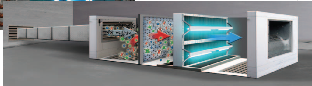
Anatomy of UVC: (clockwise) A large commercial A/C unit featuring UVC lighting; visual inspection is recommended for checking UVC systems, but not for making changeout decisions; an air-handling-system schematic shows proper location of UVC lamps at the downstream side of the cooling coil.
