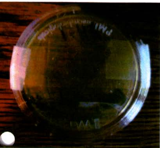
The cleanliness of the UVC-treated coils at Robbinsdale schools has been verified by petri dish testing of samples from coil surfaces.
