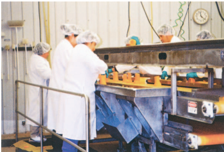
Martin Farms' butternut squash processing line is equipped with Steril-Aire UVC light.
